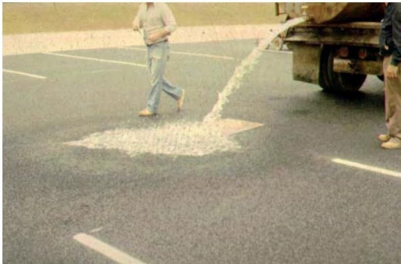
Porous Pavement Infiltration. Testing new pavement installation. Note: steady flow passes through pavement and into stone storage below with minimal spread.
