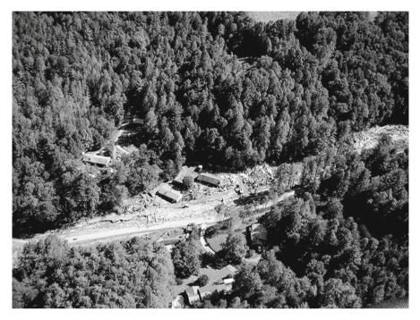
**Fig. 9.1** Damaged and destroyed homes, and debris flow erosion and deposition along the run out zone (lower track) of the September 16, 2004 Peeks Creek debris flow in Macon County, North Carolina. The debris flow triggered by rainfall from Hurricane Ivan claimed five lives and destroyed 16 homes (September 19, 2004 NCGS photo). Refer to Fig. 9.17 for location
