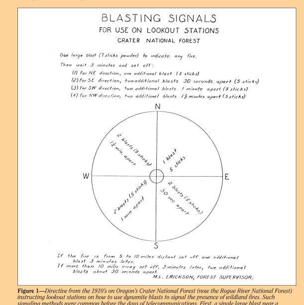
instructing lookout stations on how to use dynamite blasts to signal the presence of wildland fires. Such signaling methods were common before the days of telecommunications. First, a single large blast near a lookout station would signal the detection of a smoke. Then smaller blasts at timed intervals would signal the direction of the fire from the lookout station as well as its approximate distance.
