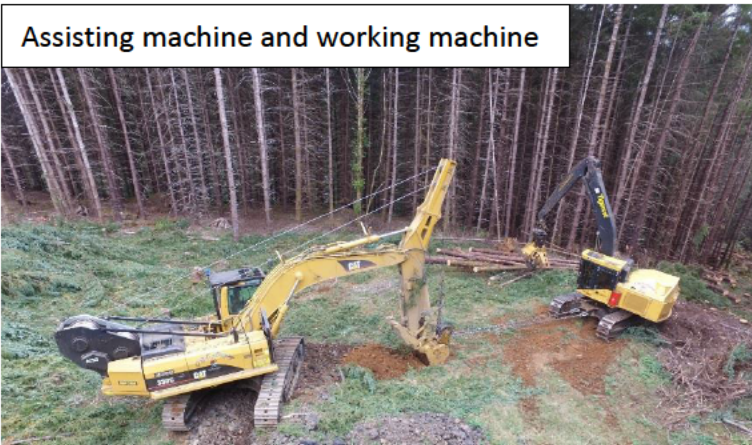
Winch mounted on working machine
