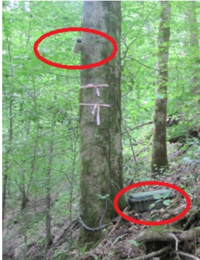
Figure 2. Acoustic set-up. The microphone is tied onto the tree and rests in PCV pipe, while the unit is chained to the tree.
