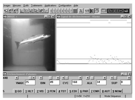
Figure 4-2. Screen image from a motion-activated fishway monitoring system Source: Travade et al. (2002)
