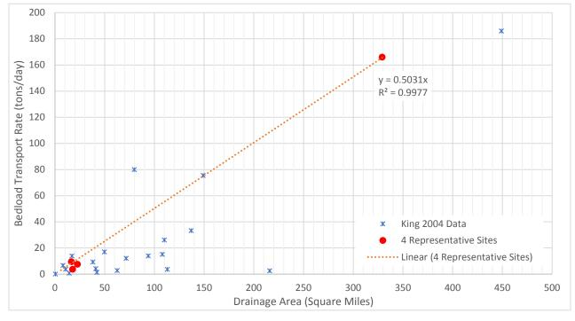
shown within these figures estimate the sediment transport rate (bedload or suspended load) associated with the bankfull discharge based on the basin area.
