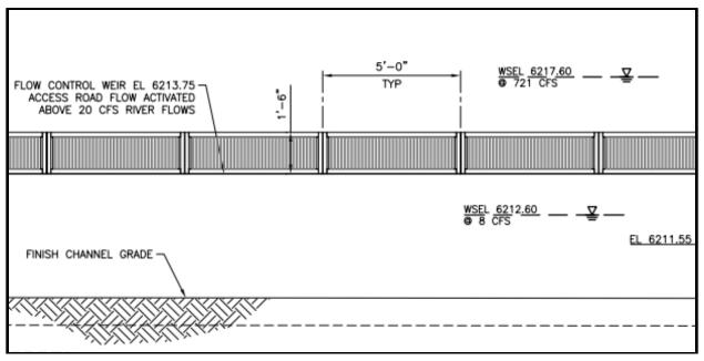
Figure 2-6. Picket panel section atop the flow control weir that would become active at streamflows greater than 25 cfs (Jensen 2019)
