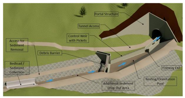
Figure 2-1. An isometric illustration of the south portal section of the EFSFSR tunnel Blue arrows indicate direction of streamflow
