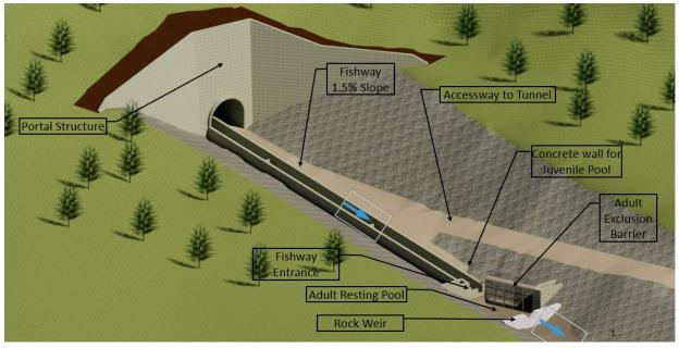
Figure 2-9. Isometric illustration of the north portal section of the EFSFSR tunnel Blue arrows indicate direction of streamflow down the fishway to the rock weir.
