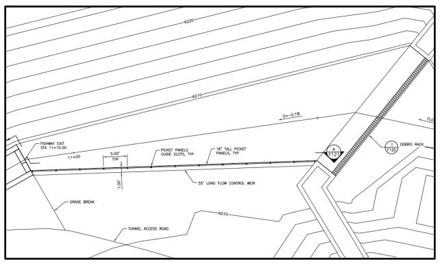
Figure 2-5. Overhead view of the flow control weir located between the debris rack and fishway
