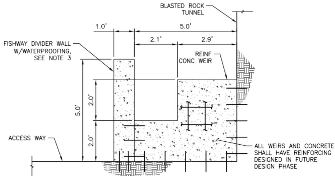
Figure 2-8. Cross-section view of the elevated fishway weir
