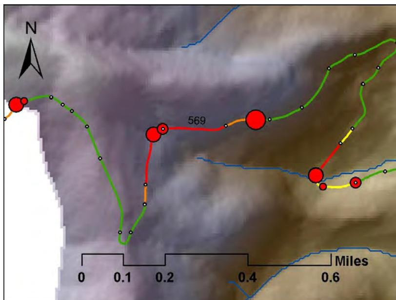
**A) NFSR 569** leading to Whitehawk Lookout has a steeper grade (9% average for displayed segment) compared to most Bear Valley roads and has the highest sediment delivery rate out of any stretch of road in the entire watershed (see Table 6).
