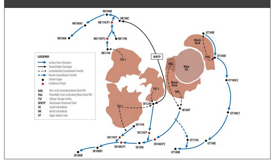
Figure 6-11. Approximate locations of stream gages and wastewater treatment plant (WWTP) discharges represented in Figures 6-8 through 6-10. Gages denoted with CP indicate confluence points, where virtual gages were created for analysis purposes. Footprint of the major mine components of the Pebble 6.5 scenario are shown for reference. Gage locations are based on U.S. Geological Survey (2012b) and Pebble Limited Partnership (2011).
