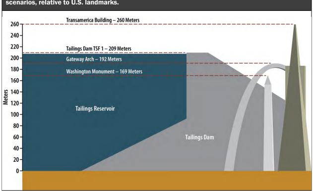
Figure ES-8. Height of the dam at tailings storage facility (TSF) 1 in the Pebble 2.0 and Pebble 6.5 scenarios, relative to U.S. landmarks.
