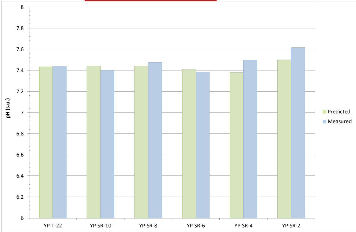
Figure 6-1: Predicted vs. Measured pH under Average Flow Conditions
