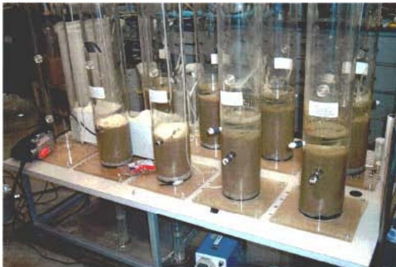
Figure 13. Eight columns set up to study four disposal scenarios for the Mount Nansen tailings
