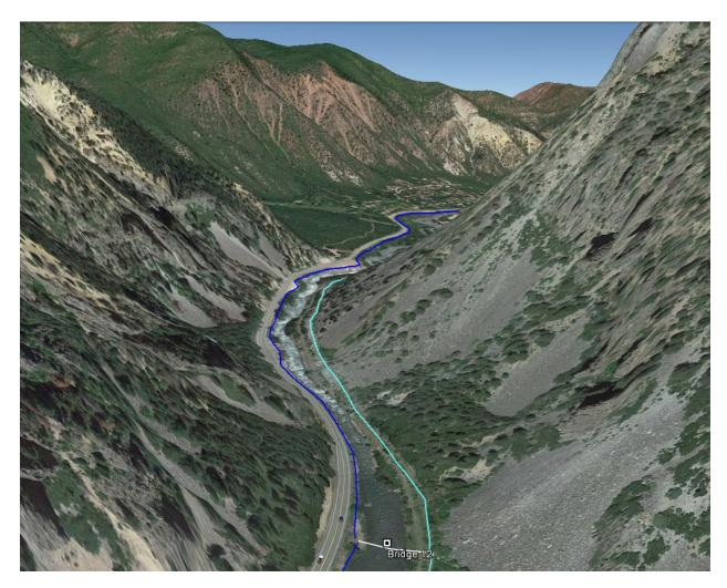
Figure 1 A typical reach through a very confined valley on the Narrows section. Encroachment and armored banks from Highway 133 (left) and the abandoned railroad (right) extend the length of this reach. Bridge option 2 is in the foreground.
