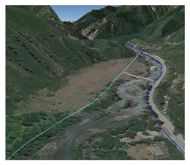
Figure 12 On the Janeway South section, riparian vegetation was cleared from the east side riparian area (left in photo) which is also disconnected from the river by the abandoned railroad line that runs though the center of the valley bottom. Routing the trail along this line in Alignment B would probably eliminate river and riparian restoration potential on this impaired reach.
