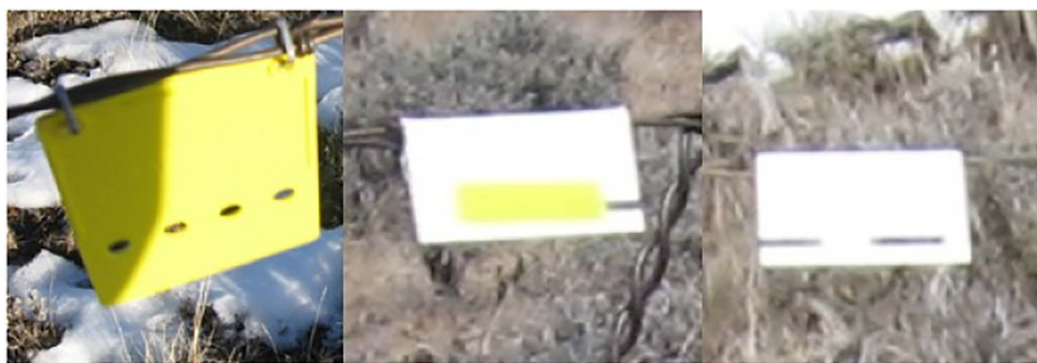
Fig. 2. Photographs of fence marker types deployed in our study. From left to right the above images represent the Flysafe, reflective, and white marker treatments.
