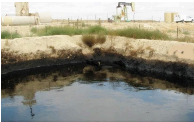
During production, the process of separating oil and produced water using heat treaters is often ineffective. The produced water is either discharged into surface waters, injected underground, or
