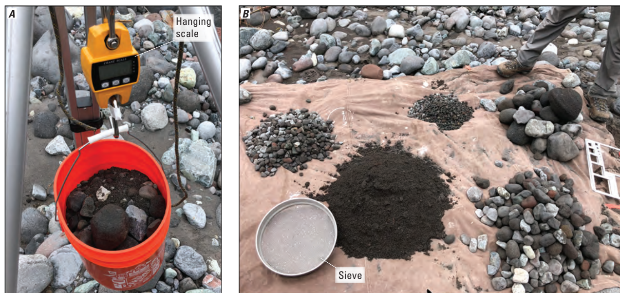
Figure 7. In situ set up of field weighing (A) and sieving (B) subsurface bulk sediment sampling.
