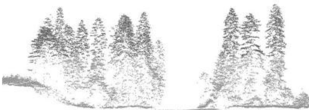
Fig. 2. LiDAR point cloud illustrating the 8-point per square meter resolution of the data in a riparian forest stand in southeast Alaska, USA, collected in summer 2017.
