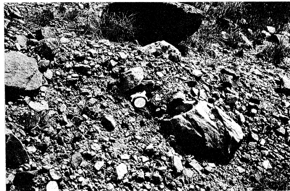
Figure 18 - Track Etch Detector Placed on Spoils Pile.
