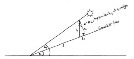
$A_s$  = sun angle above the horizon, not the ground surface,  $h_1$  = height of the line drawn from the tree tip, perpendicular to the ground, and  $d_1$  = distance from interception of that line with the ground, to the base of the tree.
