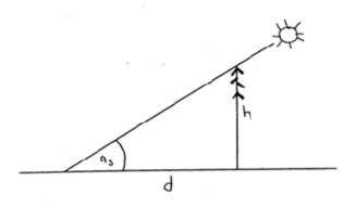
A<sub>s</sub> = sun angle, h = tree height, and d = shadow distance
