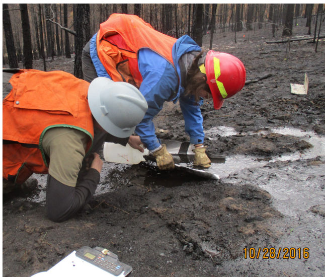
FIGURE 4 The rill flow being collected with a flexible aluminium sheet in the main rill about 15 m from the inlet at Cayuse Mountain site 2-month post-fire
