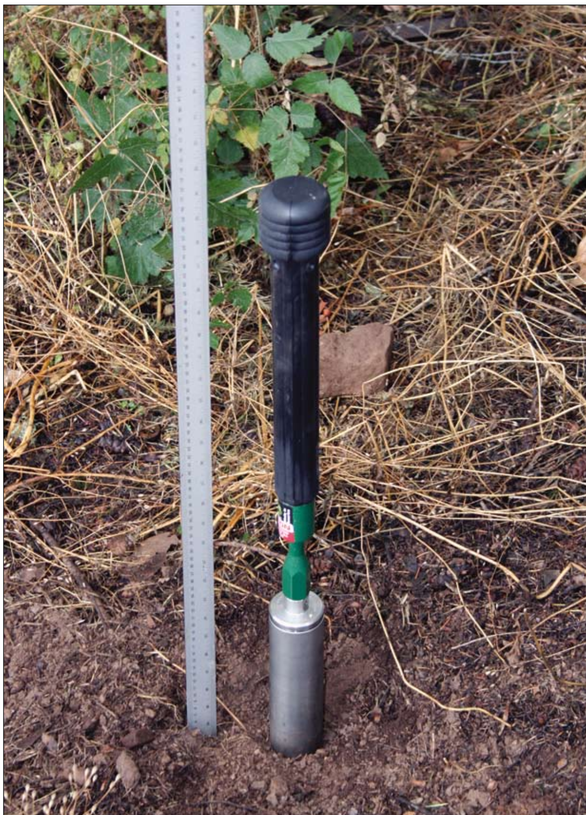
Figure 55—Forest soils are sampled with a soil coring device driven by an impact hammer.
