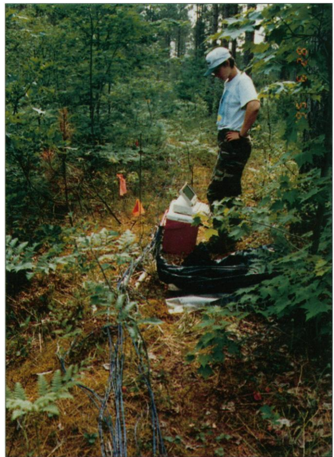
Figure 8. Multiple microclimatic variables are measured concurrently every 5 m along a 760 m transect in the Chequamegon National Forest, northern Wisconsin.
