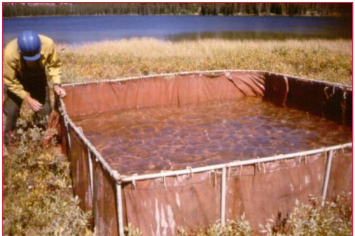
**Figure 1**—A 5,944-quart (5,625-L) fold-a-tank storage facility near the inlet to Bull Trout Lake, Boise National Forest, ID. After dipping the helibucket into small, high-elevation lakes, the pilot released the water into the tank. Researchers then searched the water for captured fish during a study on the potential removal of threatened, endangered, and sensitive fish species through helibucket dipping. Photo: Justin Jimenez, USDA Forest Service, Boise National Forest, Boise, ID, 1999.
