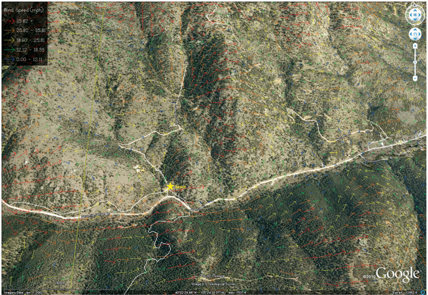
Figure 19. Wind directions displayed (modeled) using the WindWizard software for the Fourmile Canyon Fire focusing on where the fire started near the mouth of Emerson Gulch. Note the faster winds (red) blowing along the ridges.
