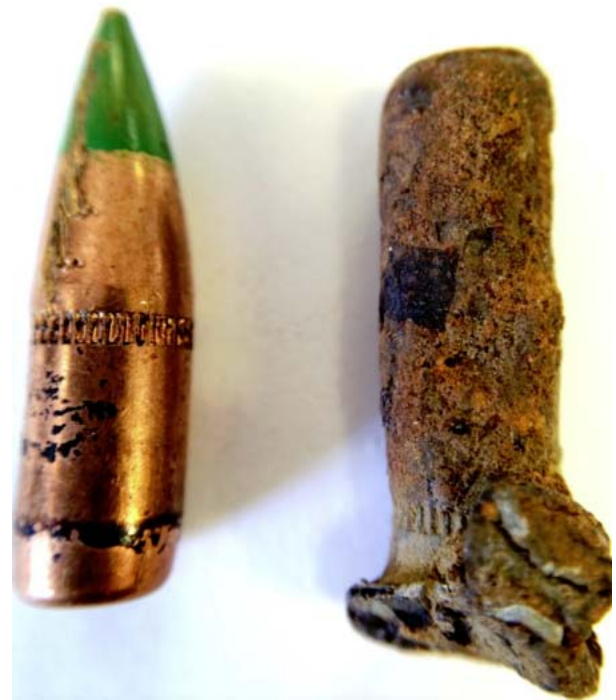
Figure 3. Optical images of a new 5.56mm bullet (left) and a 5.56mm bullet that weathered for 15 years (right). The tip of the bullet fragmented and the weathering crust can be hundreds of microns thick and comprised of secondary mineral phases. Photo by A.J. Barker.
