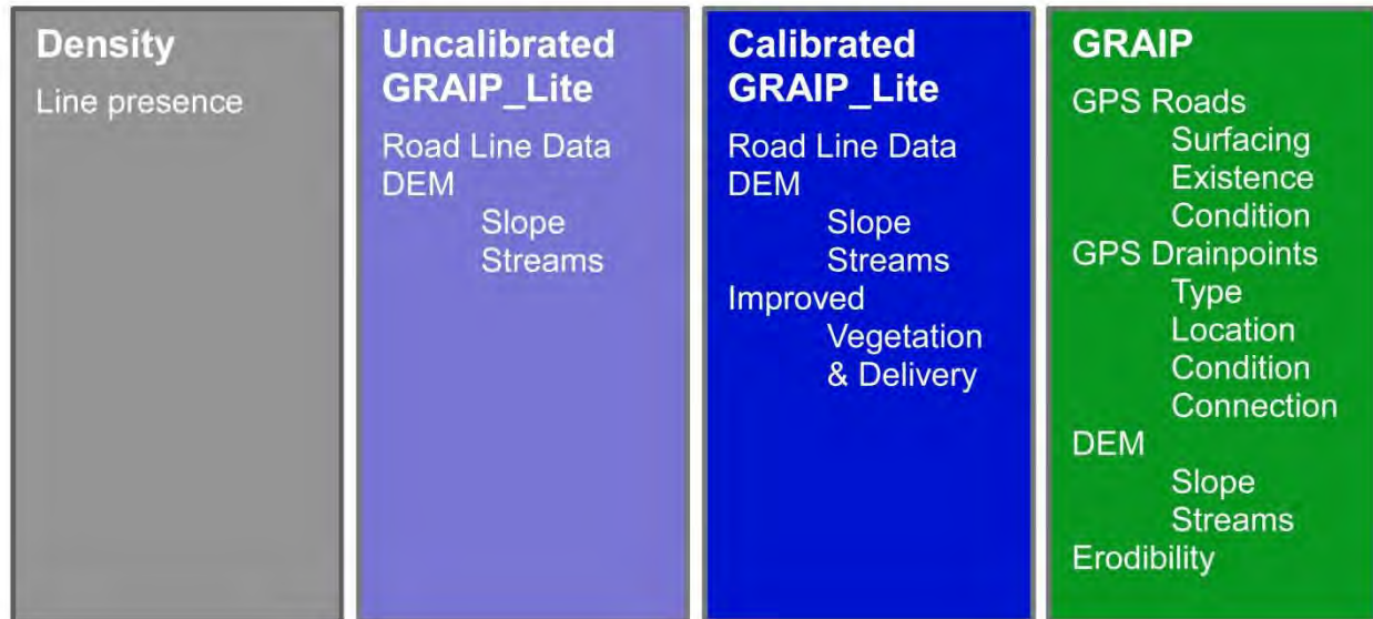
Figure 1: The information-effort scale for road erosion estimation.
