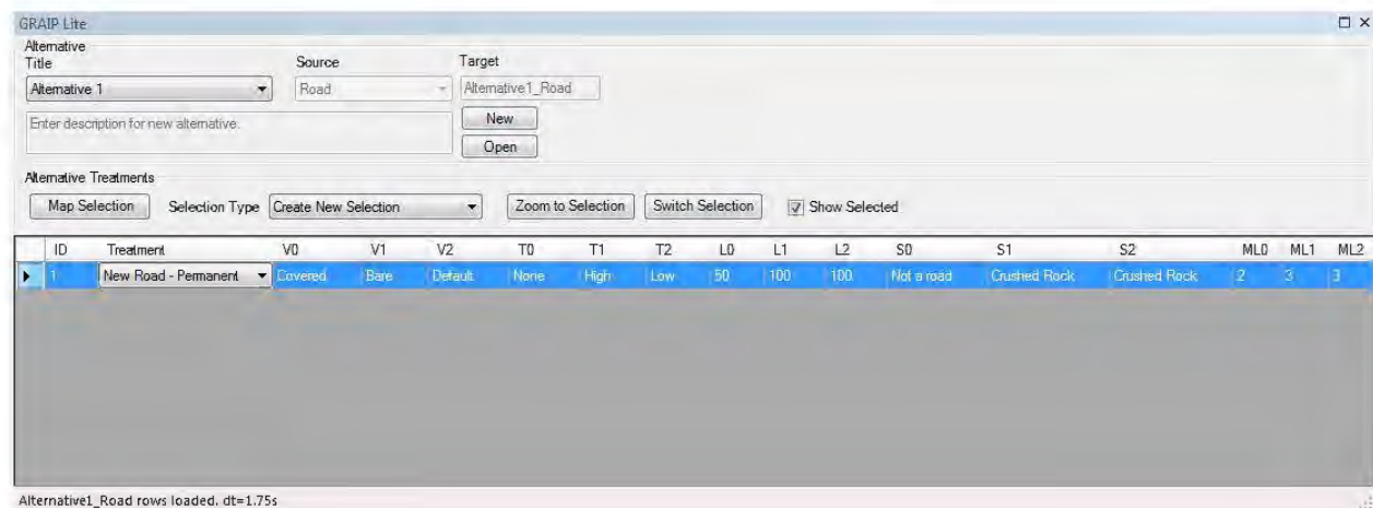
Figure 65: Assign treatment; note that S0 , the surface factor for the initial condition, is set to “Not a road”.
