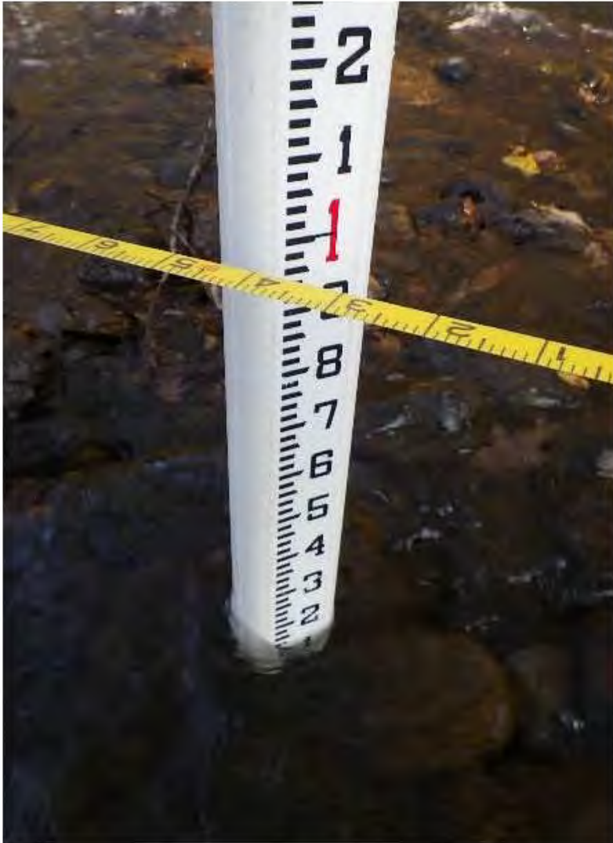
Figure 5. Detail of stadia rod used to measure depth along a critical riffle transect
