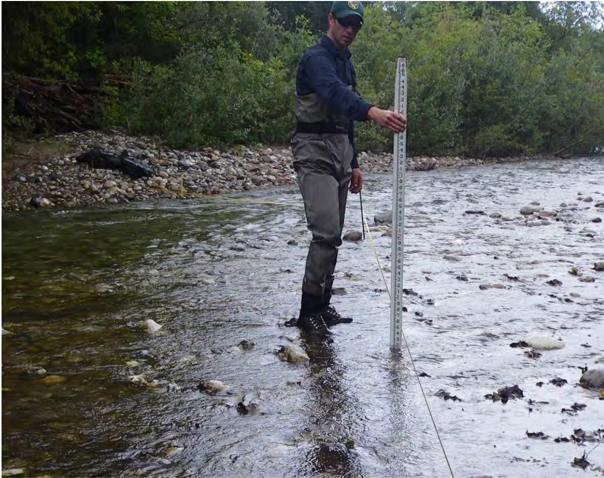
Figure 4. Example using stadia rod to measure depth along a critical riffle transect
