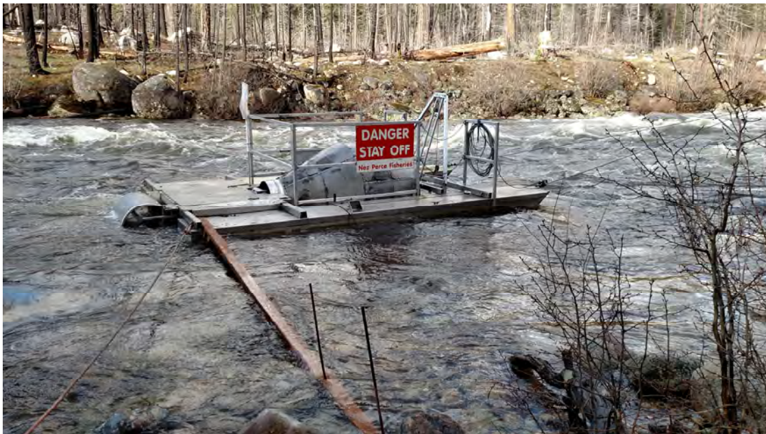
Appendix Figure 6. Rotary screw trap located on the lower Secesh River used for capturing migrating juvenile Chinook salmon.
