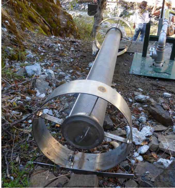
Figure 8-10 Typical end-of-pipe screen equipped with “wagon wheels” to elevate the screen off the stream bottom
