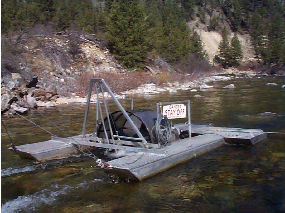
Appendix Figure 5. Rotary screw trap located on Johnson Creek used for capturing migrating juvenile Chinook salmon.
