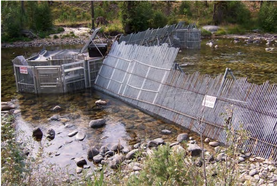
Appendix Figure 4. Adult picket weir, upstream trap box, holding and workup area located on Johnson Creek used for capturing Chinook salmon.
