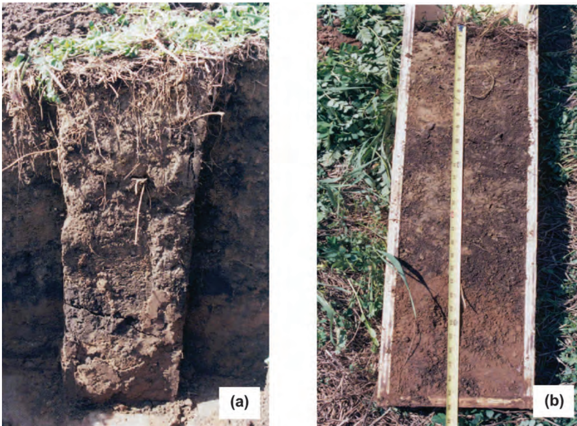
Fig. 4. (Color) (a) Soil-root monolith on the wall of trench; (b) monolith trimmed into sample box. Surface of GCL is visible at the bottom of the trench in (a).
