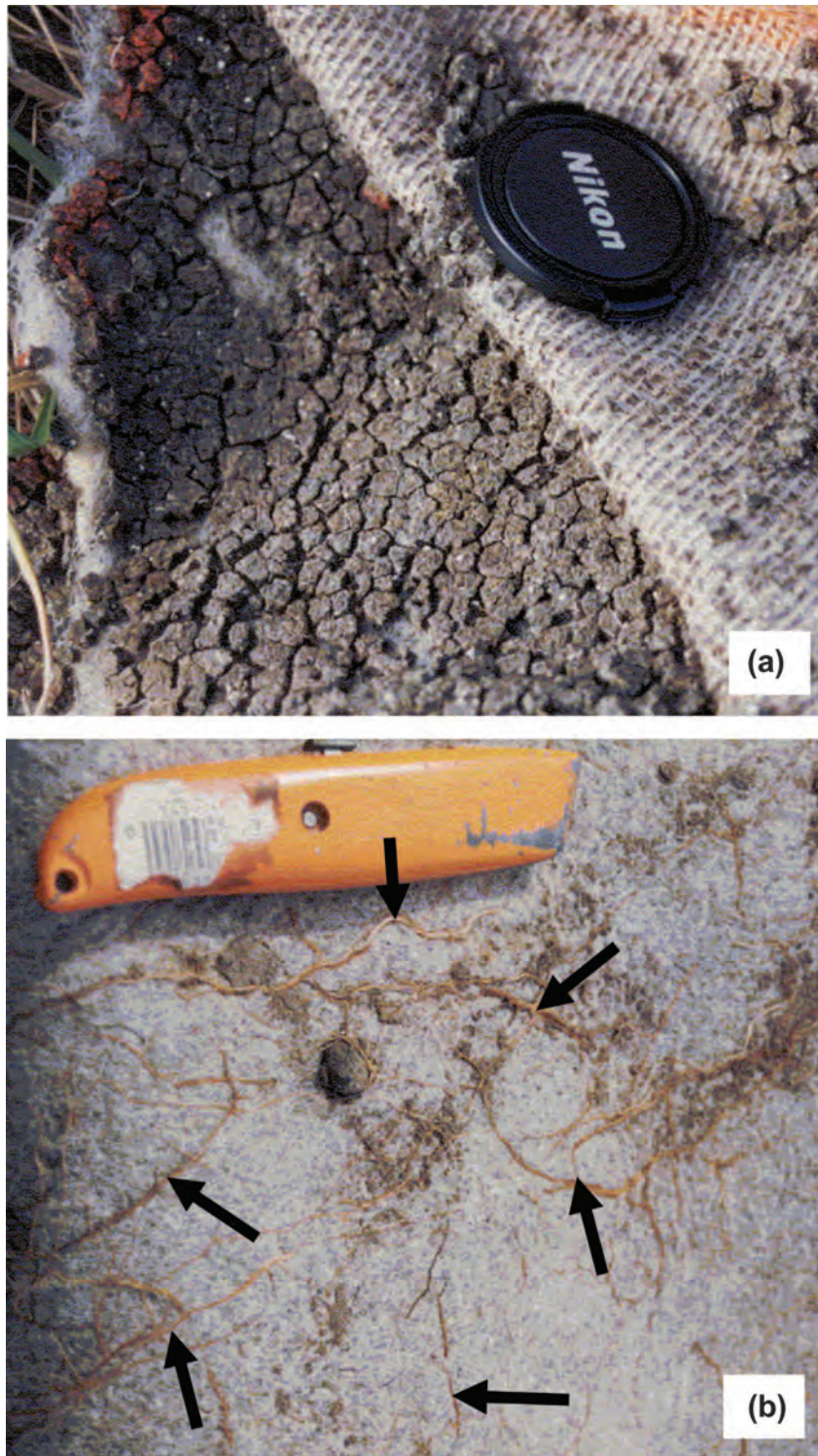
Fig. 3. (Color) Observations made during second reconstruction of Lysimeter 2: Desiccated and cracked bentonite (a); roots penetrating to underside of GCL (b)
