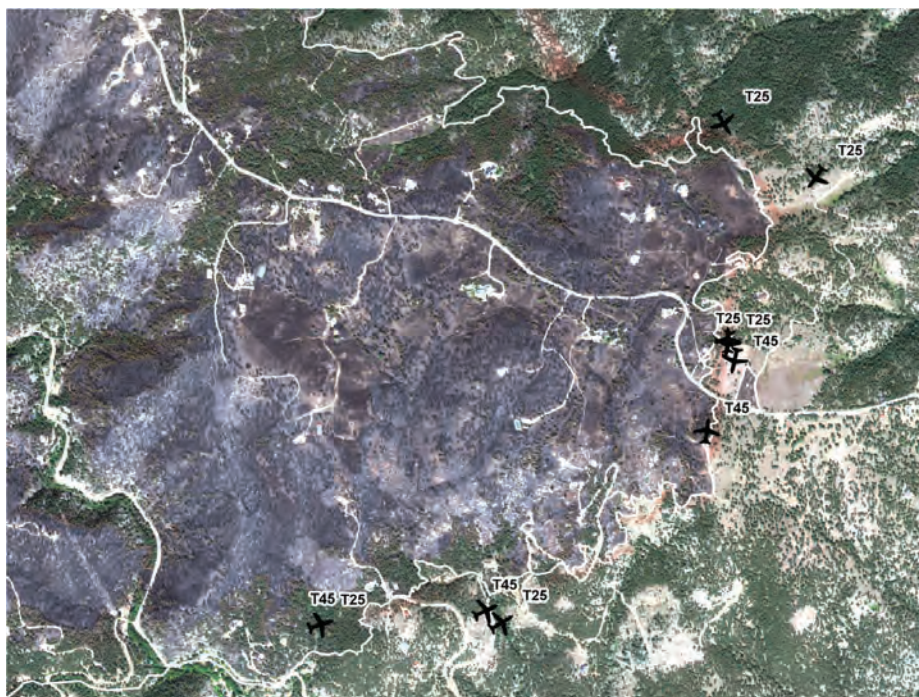
Figure 39. Top photo shows tanker T-25 heading towards the Bald Mountain Open space area on September 6, 2010 at 1800 hours (photo: Mark Leffingwell, Denver Post). Bottom image shows drops made in the Bald Mountain and Camino Bosque/Arroyo Chico area on September 6, 2010. Red areas along the fire edge are fire retardant. The white line shows the final fire perimeter on September 17, 2010. Background is a WorldView satellite image from Digital Globe taken September 12, 2010 at 1159.
