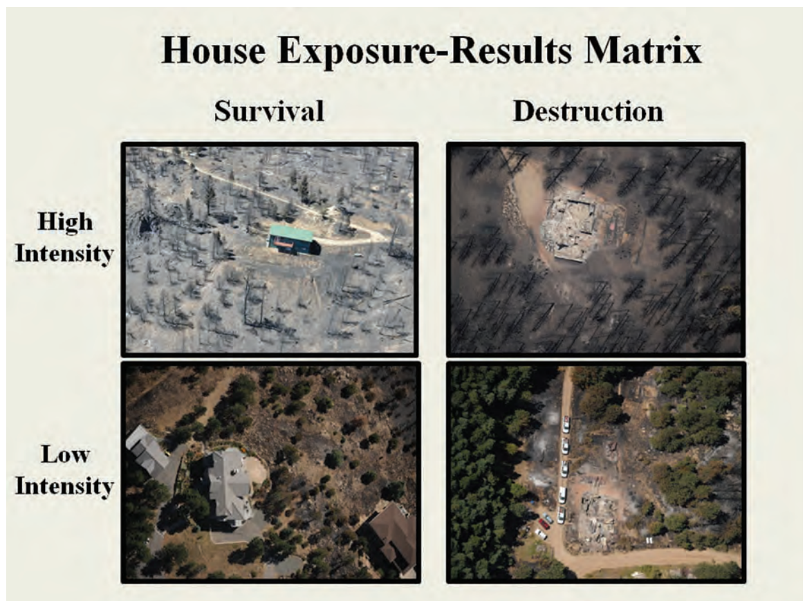
Figure 56. Home destruction and survival are associated with both high and low intensity fire exposures. Most destroyed homes (139, 83%) in the Fourmile Canyon Fire occurred with low fire intensities in the home ignition zone (HIZ) (photo: Dave Zader (upper left); Joe Amon (all others)).
