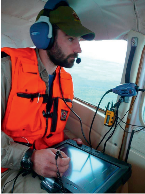
FIGURE 14.2 Digital sketch-mapping systems are now commonly used during aerial survey. The system, consisting of a tablet PC, external GPS receiver, and stylus, has the capability to display multiple types of background images for navigation and mapping (aerial imagery, topographic maps, etc.) and vector data (e.g., administrative and political boundaries, aerial hazards, etc.). Photo credit: D. Wittwer, Forest Health Protection, USDA Forest Service.
