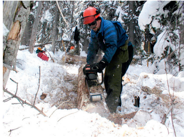
FIGURE 14.4 Log Wizard™ being used to peel bark from Picea engelmannii infested with Dendroctonus rufipennis in Utah, United States. This and other similar methods are often used in conjunction with sanitation and trap tree methods to destroy brood and adults beneath the bark. Photo credit: S. Munson, Forest Health Protection, USDA Forest Service.
