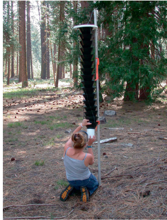
FIGURE 14.8 An attractant-baited multiple-funnel trap used for monitoring bark beetle populations. Photo credit: C. Fettig, Pacific Southwest Research Station, USDA Forest Service.
