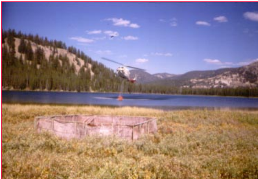
Figure 2 —Helibucket dipping with a short line and dip tank. Note the rotor wash. Researchers on the Boise National Forest believe that fish avoid helibucket dipping from a short line probably because of rotor wash. Photo: Justin Jimenez, USDA Forest Service, Boise National Forest, Boise, ID, 1999.
