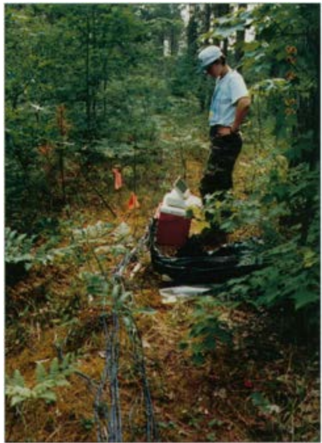
Figure 8. Multiple microclimatic variables are measured concurrently every 5 m along a 760 m transect in the Chequamegon National Forest, northern Wisconsin.
