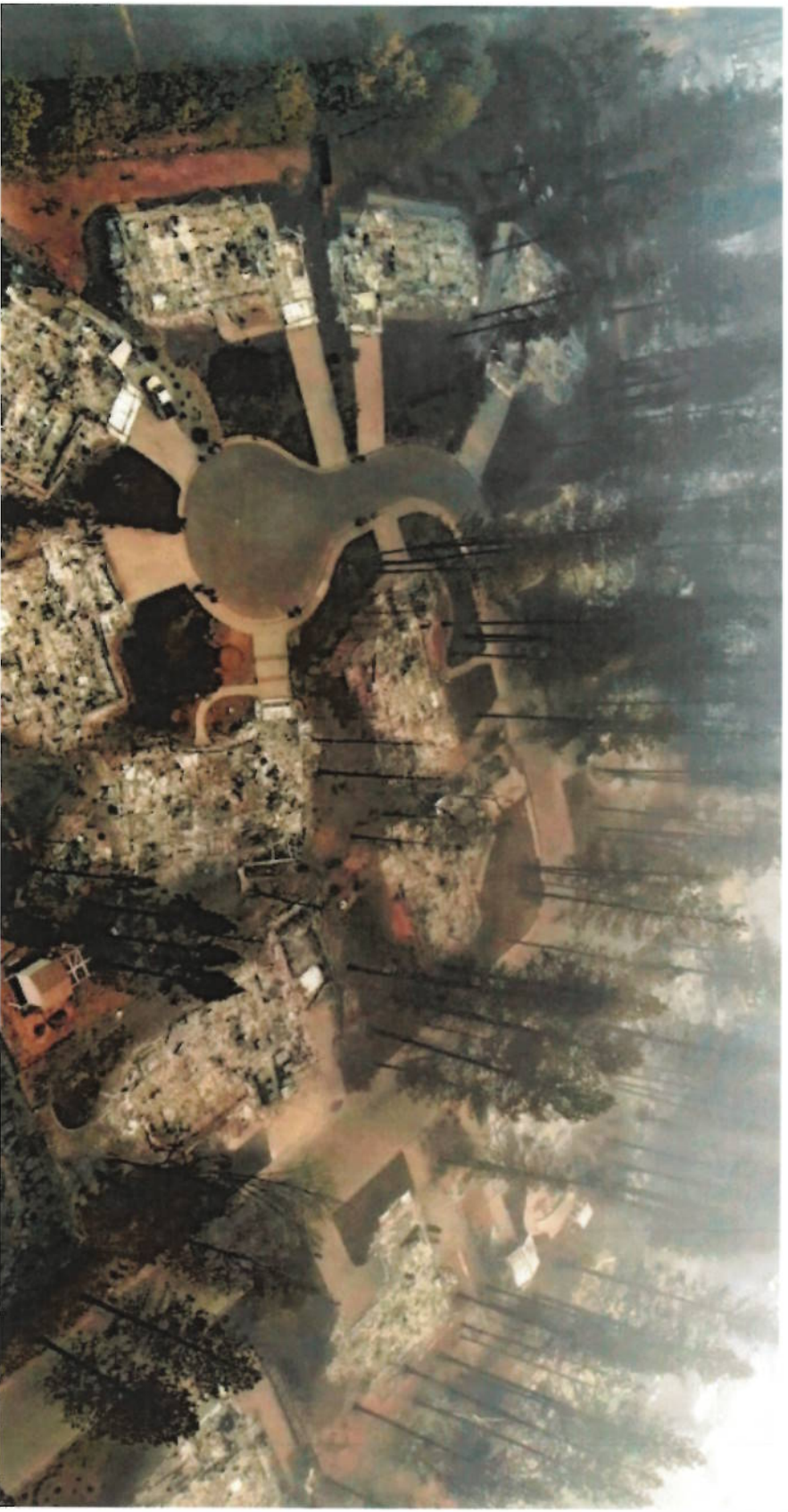
2018 Paradise Ck. — note standing green trees adjacent to burnt structures
