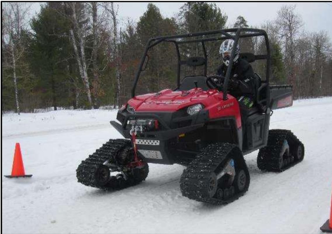
**Photo 7: OHV 2 (UTV) – Polaris Ranger 700 with Camoplast tracks, front view**
