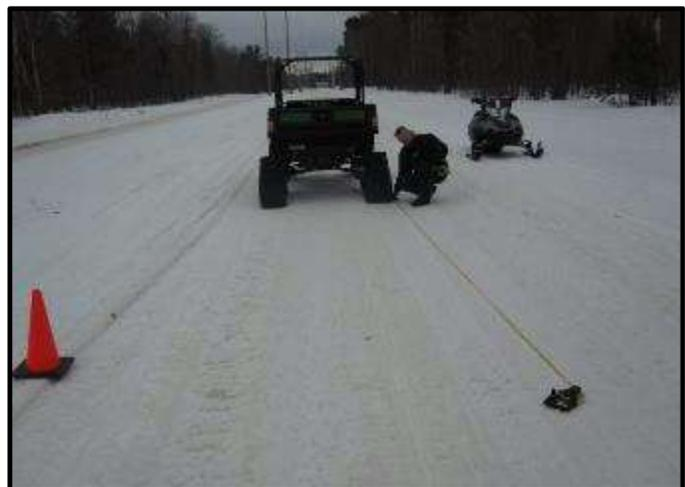
**Photo 27: Measuring Vehicle Stopping Distance**
