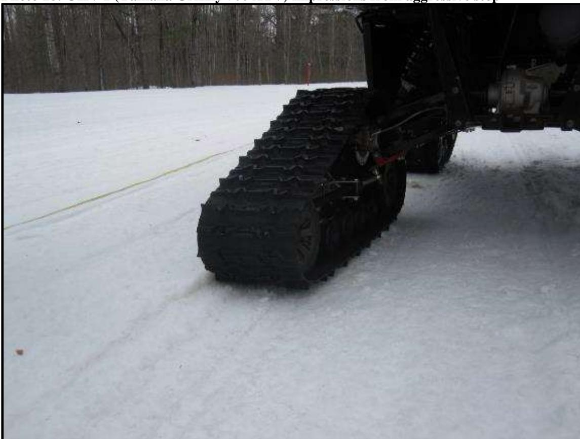
**Photo 19: OHV 2 (Polaris Ranger 700 UTV) impressions from aggressive stop**
