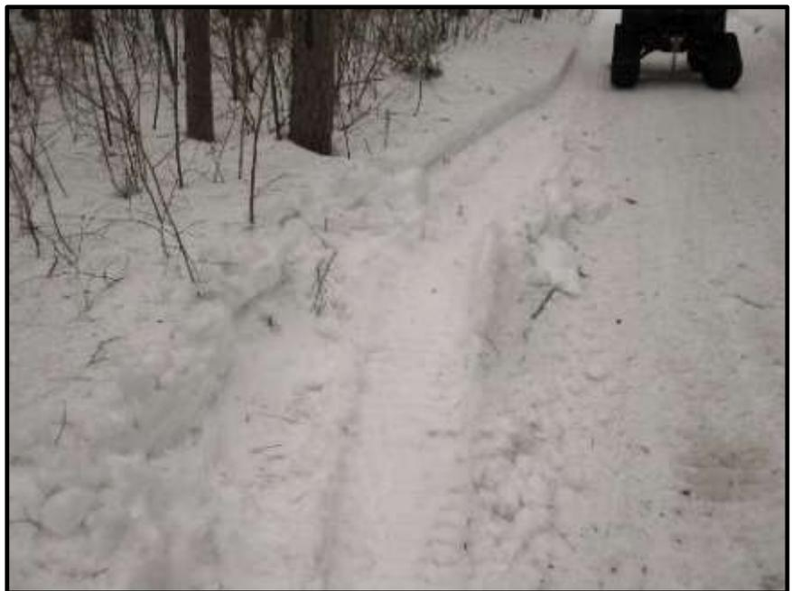
**Photo 28: Tracked OHVs were able to operate okay with one track off the compacted trail base**
