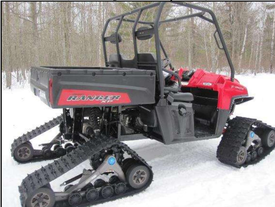
**Photo 8: OHV 2 (UTV) – Polaris Ranger 700 with Camoplast tracks, side view**
