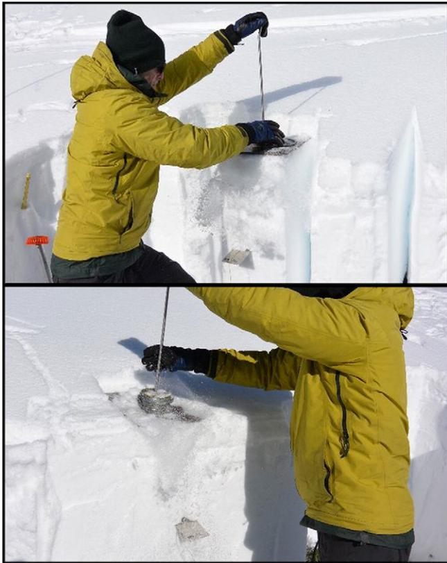
Fig. 2. The drop hammer test experiments being performed. The top shows the test configuration where the column is isolated, whereas the bottom shows the less disturbed snow cover test configuration.
