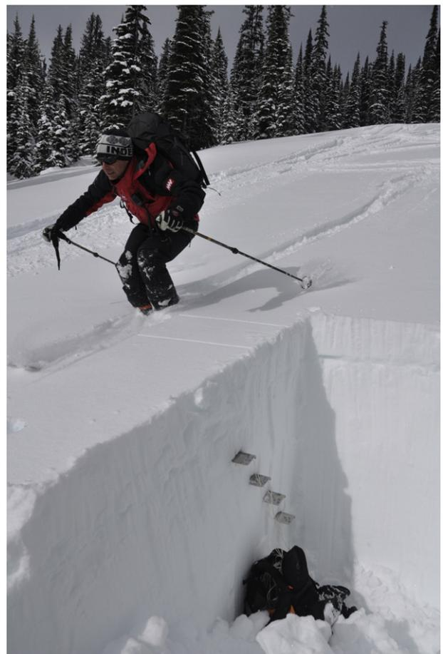
Fig. 1. Skier performing an experiment loading the snow surface above the buried sensors.
