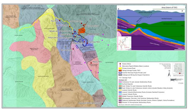
Figure 7. Cross-section B-B shows the Taylor Fault that runs through the mine. (from MPO Fig 112, p. 3-25)
