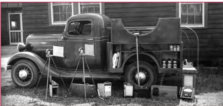
Vehicle and equipment used in fire behavior studies by fire research staff of the Southern Forest Experiment Station during the mid to late 1930s on the Harrison Experimental Forest, De Soto National Forest, MI. From left to right, the instruments are Foxboro pyrometer, thermocouple wire, thermocouple switch dial, storage battery, compass and Jacob staff, 8-pen thermograph recorder, portable recording hygro-thermograph, hand aspirated psychrometer, anemometer, and wood carrying case. In the truck compartments there are glass jars for fuel samples, cans for soil samples, a chain, and cloth of varying colors for plot markings. Photo: T.T. Kohara, Forest Service, 1937.
