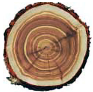
Figure 11 —Cross-section of western redcedar showing the ‘archery target’ pattern colour variation found in some interior areas of BC and the northwestern United States. (Disk supplied by Pope & Talbot, Grand Forks, BC. Text and image sourced from Gonzalez 2004).
