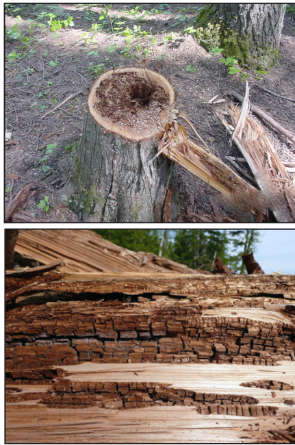
Figure 14 —Brown cubical rot in western redcedar caused by Postia sericeomollis .
