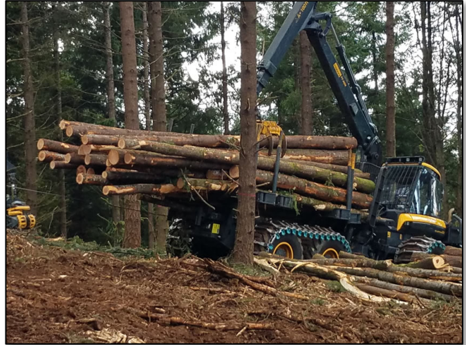
Figure 29: Tethered Forwarder on a steep slope harvest. Photo by Lisa Ball, Pacific Northwest Region, US Forest Service. Photo credit: USDA Forest Service.
