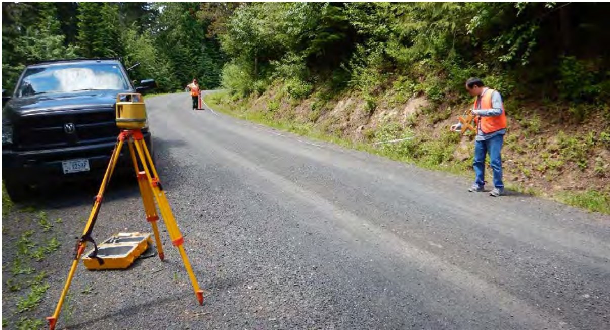
Figure 5. Measuring the length and steepness of a road segment in the Clear Creek Watershed in June, 2017, to support the development of a GIS topographic analysis technique for analyzing the larger road network.
