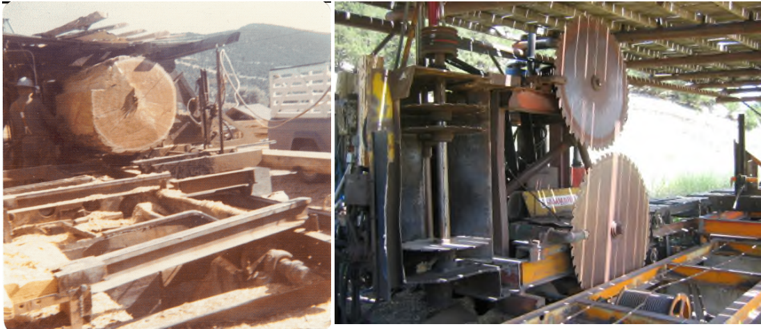
Sawing big Douglas Fir – 1974 Detail of Sawmill with top saw and vertical edger
