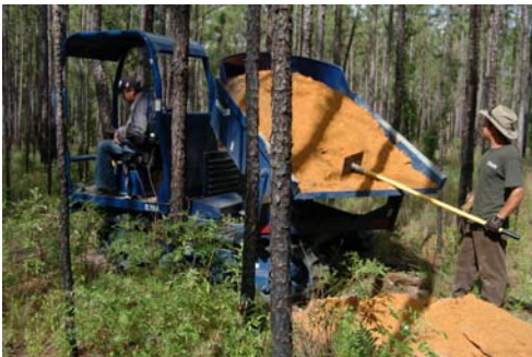
Rubber tracked haulers employed to move materials on trailbuilding projects
