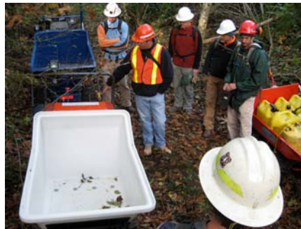
Rubber tracked haulers employed to move materials on trailbuilding projects
