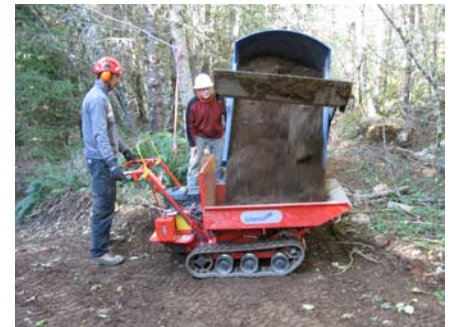
Rubber tracked haulers employed to move materials on trailbuilding projects
