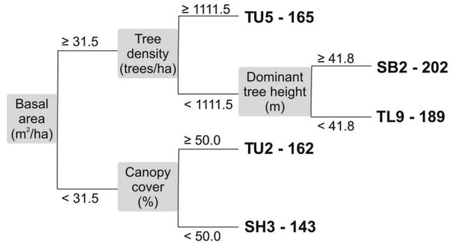
**Figure 2.** Surface fuel model selection logic for Last Chance stands. This logic did not apply to all treated stands in 2017 or to thinned/prescription-burned stands in 2027. The break values for the logic were determined from three separate regression tree analyses (see Methods for explanation). Surface fuel models were selected from Scott and Burgan (2005) and are identified in bold by code and number.
