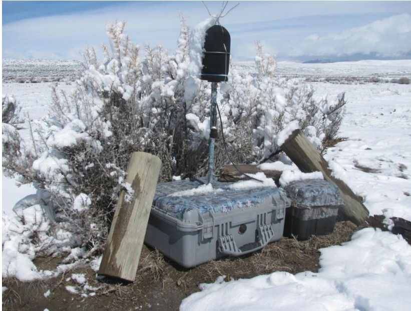
Fig. 2. Sound level meter (SLM, on left) and audio recorder (SM-2 Wildlife Acoustics, on right) deployed in field on a Gunnison sage-grouse lek, in the Gunnison Basin, Colorado, spring 2013.
