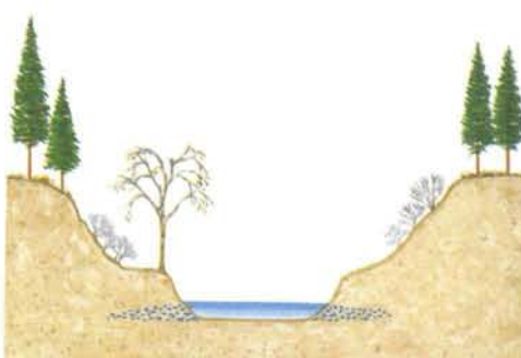
Stream channel widens and shallows in response to deteriorating upland and/or riparian conditions
