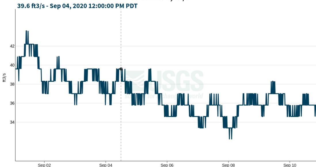
The graph shows the early September hydrograph in exquisite detail, clearly showing the contribution of evapotranspiration to streamflow in late summer, at the USGS stream gage near Twisp on the Twisp River. Look closely at the timestamp and the vertical line that indicates time of day.
