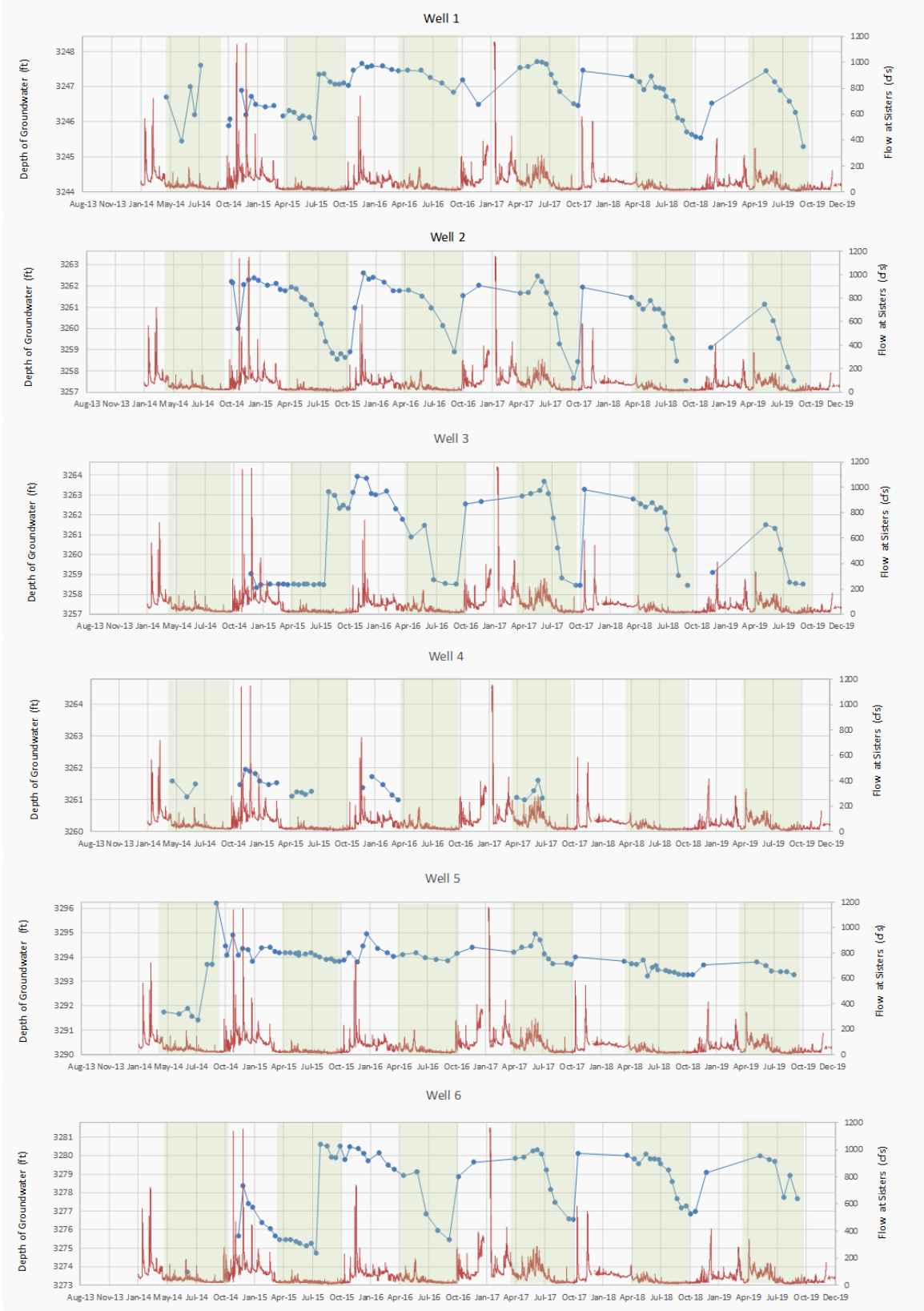
Figure 22. Groundwater well monitoring from Whychus Floodplain Project with the mean daily flow (red line) of Whychus Creek at Sisters plotted on the right vertical axis. Growing seasons are shaded green.
