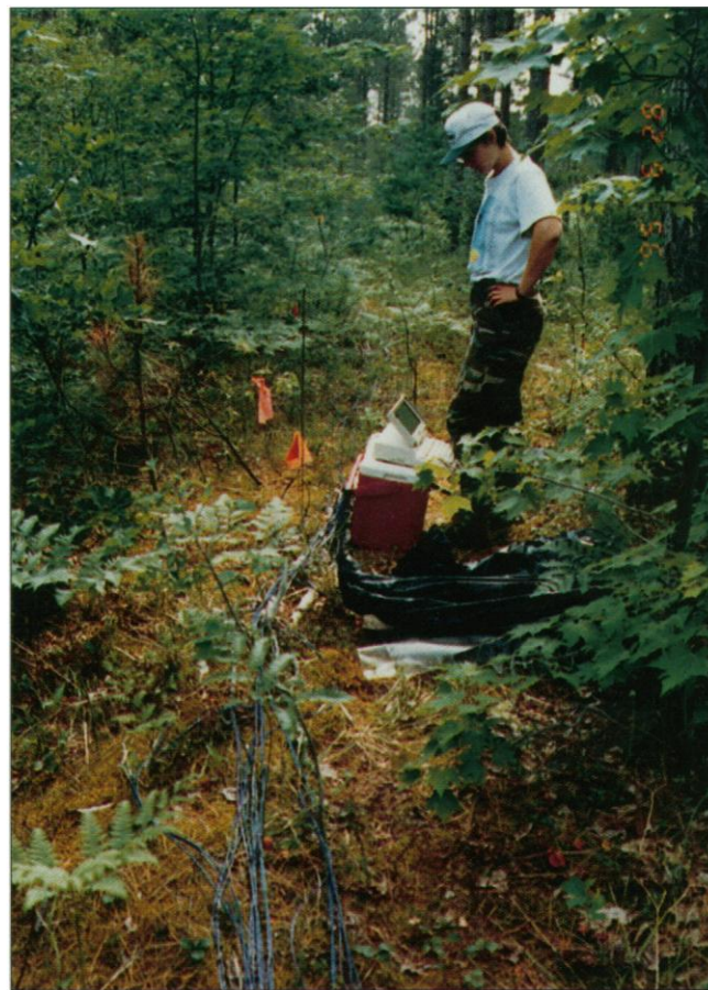
Figure 8. Multiple microclimatic variables are measured concurrently every 5 m along a 760 m transect in the Chequamegon National Forest, northern Wisconsin.
