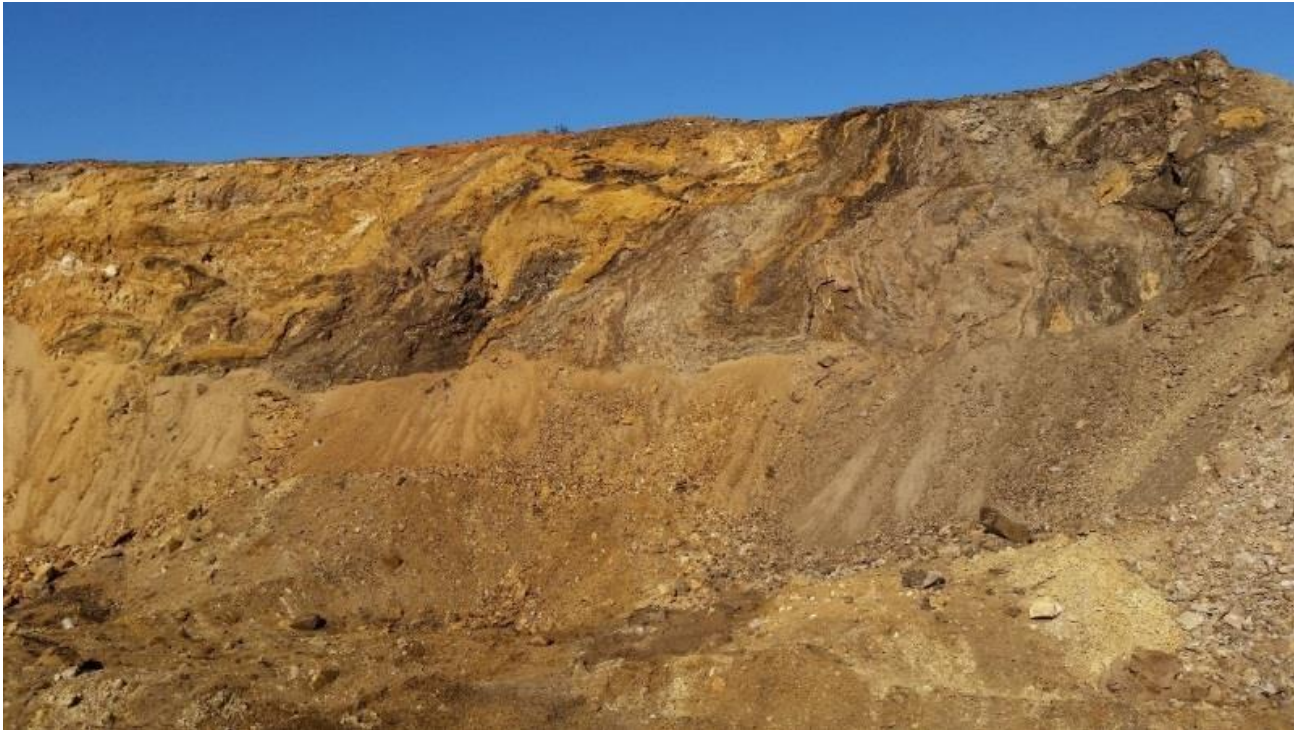
Figure 22. West wall of Castle Sands Company Quarry (mined by Titan America) showing rip-up and deposit of alluvial fan. Material is friable and somewhat sorted. Black material shows concentration of coating around a “ball” of rip-up rock. The rip-up rock has weak single grain structure but is pulverized and held in place by the matrix of yellowish brown material (slightly shaly, platy) (photo by author, 2015)
