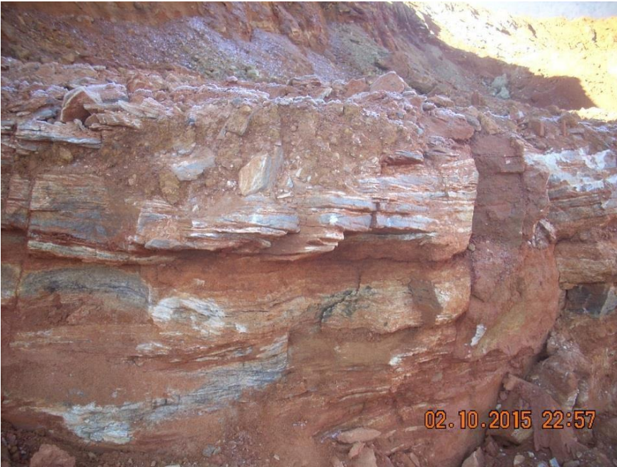
Figure 18. This is the quarry rock being mined in the south view in above photo. It is considered Rocky Gap (Ridgley) Sandstone (Froehling & Robertson, 1990). Ridgley sandstone in photo is quite friable (photo by author, 2015).
