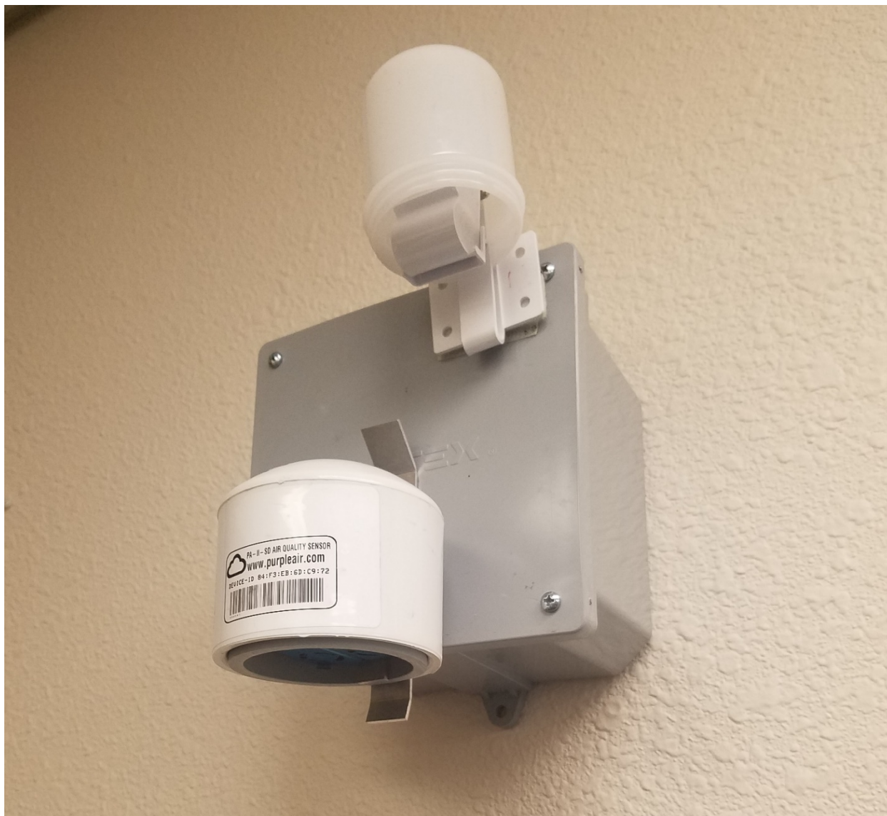
Figure 4. PurpleAir unit and Ogawa SO 2 passive sampler attached to the junction box housing.
